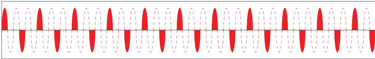
The advantage of AFC over burst is the reduction in thermal cycling. Another advantage of AFC is that visual flicker is less noticeable than distributed thus making it suitable for shortwave infrared heater applications.
