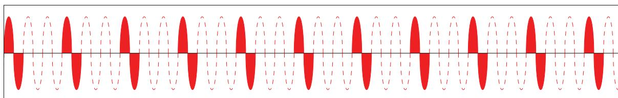
The advantage of distributed over burst is the reduction in thermal cycling. On the other hand, distributed suffers from worse harmonics/emissions than burst.
