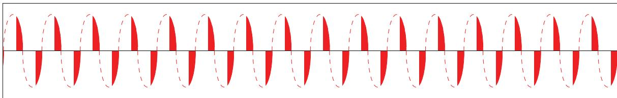
The advantage of phase angle over the other switching modes is its precise resolution of power. However, phase angle generates excessive harmonics vs other switching modes. With phase angle control, the flickering of IR heaters is eliminated completely.
