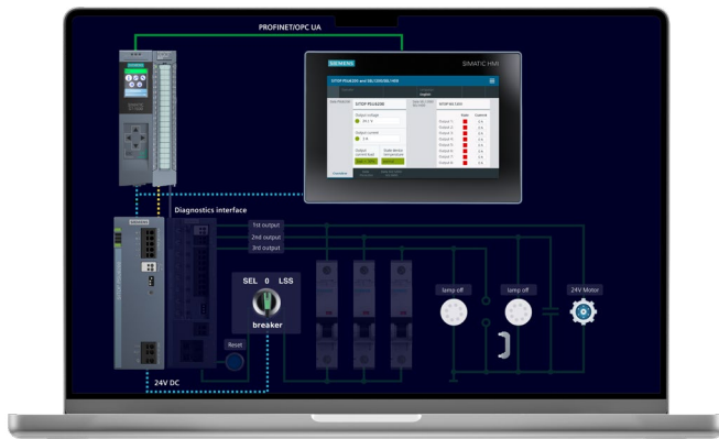
Virtual demo model with SITOP PSU6200 and SITOP SEL1200
